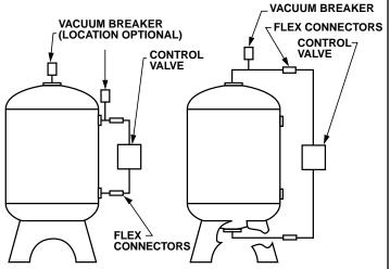
NOTE: Flexible connectors must be installed between hard piping and tank openings. These pressure vessels are rated for an internal negative pressure of 5<sup>°</sup> HG (17 Pa) vacuum below atmospheric. If negative pressure could ever exceed 5<sup>°</sup> HG (17 Pa), an adequate vacuum breaker must also be properly installed. Failure to install flex connection properly, or improper installation of a vacuum breaker when required, may void the warranty.
