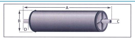
Model Weight Part Numbers inches (mm) inches (mm) inches (mm) lbs (kg) Interconnector O-ring Brine Seal 0035458 0035702 4040-SW 40 (1,016) 4 (101.6) 0.75 (19.0) 1.0 (25.4) 10 (4.5) 0035267
