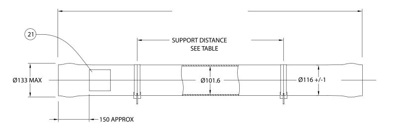
Working Pressure: 600 psi Working Temperature: 0° to 45°C
