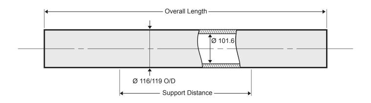
Working Pressure: 300 psi Working Temperature: 0° to 45°C
