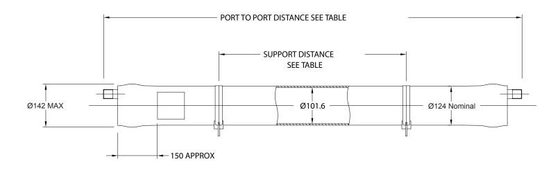
Working Pressure: 1200 psi Working Temperature: -70 to 450C
